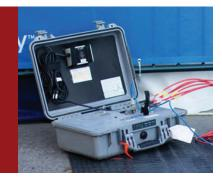
The MyLaps system consists of a decoder and antennas that read the chips. For most events, we use hard rubber mats that house antennas that lie flat on the ground, so athletes do not trip as they cross. Side Antennas are used when ground mats are not feasible, such as for some bicycling races, and Nordic ski and snowshoe races.
